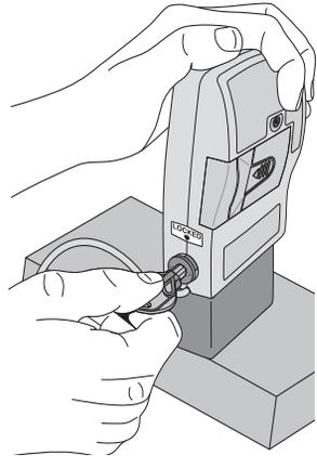
4. Insert the key into the lock, push in, and turn counterclockwise until the line on the lock lines up with the arrow on the side of the pump and you feel the lock click into place.
