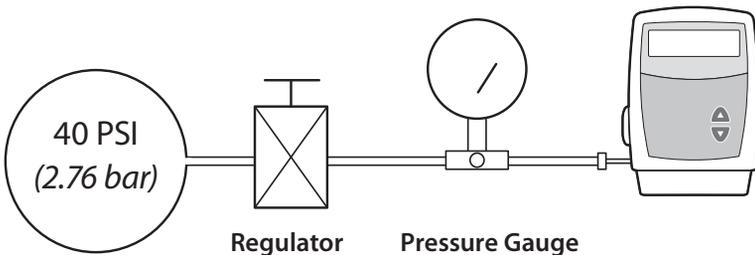
4. Connect the CADD™ medication cassette reservoir outlet tube to the metered pressure source.
