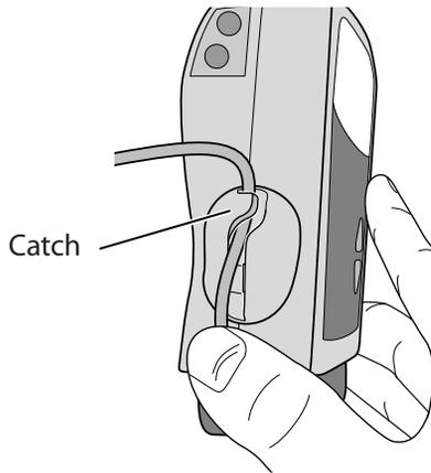
3. To seat the tubing into the groove, gently pull the tubing, until it is under the retention nubs and flat in the groove.
