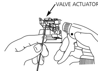
**NOTE:** A broken valve actuator tip may be supported by the actuator seal and may not appear defective.
